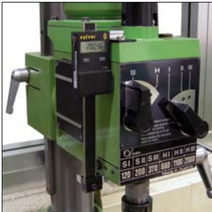
Depth measurement on a drilling machine
