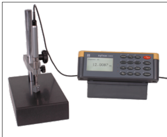
Measurement of 4 sizes on 4 channels with one single probe
