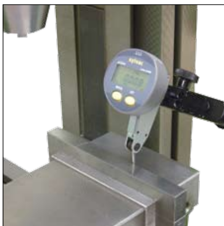
Checking the alignment of a vice on milling machine.
