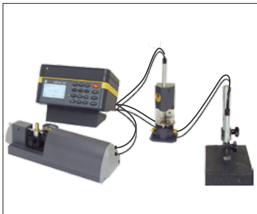
Using 3 measuring channels with 3 separated probes
