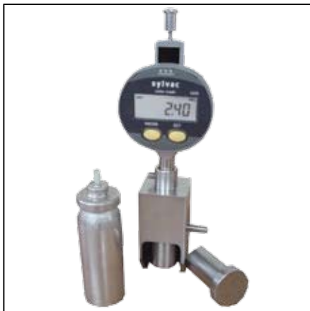
Checking of an internal \varnothing with a mechanical head
