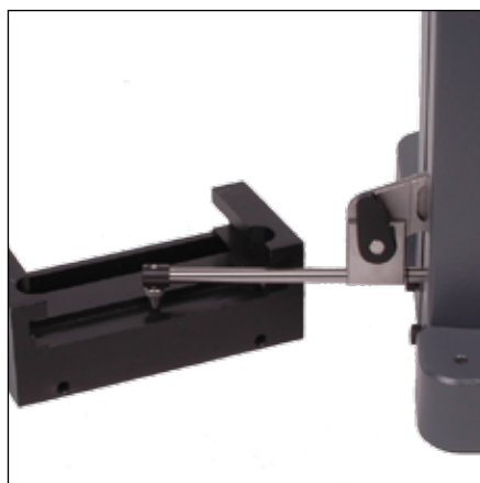
Depth measurements with accessories 930.2108 and 905.2204
